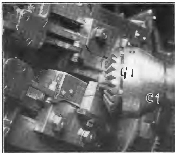
Fig. 6—Gleason planer profiling bevel gears after they have been gashed in the milling machine
